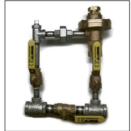
Product Note: The Viking Model D-2 Air Pressure Maintenance Device, preassembled with bypass trim (Viking Part Number 07459), provides the necessary isolation valves, union, and bypass trim valve. Refer to Figure 1.
